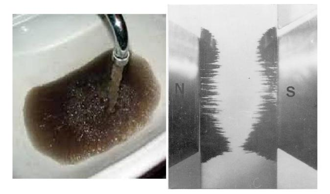
Figure 6. Photograph of the ferromagnetic admixtures filtered from passing water in the gap of electromagnetic device
