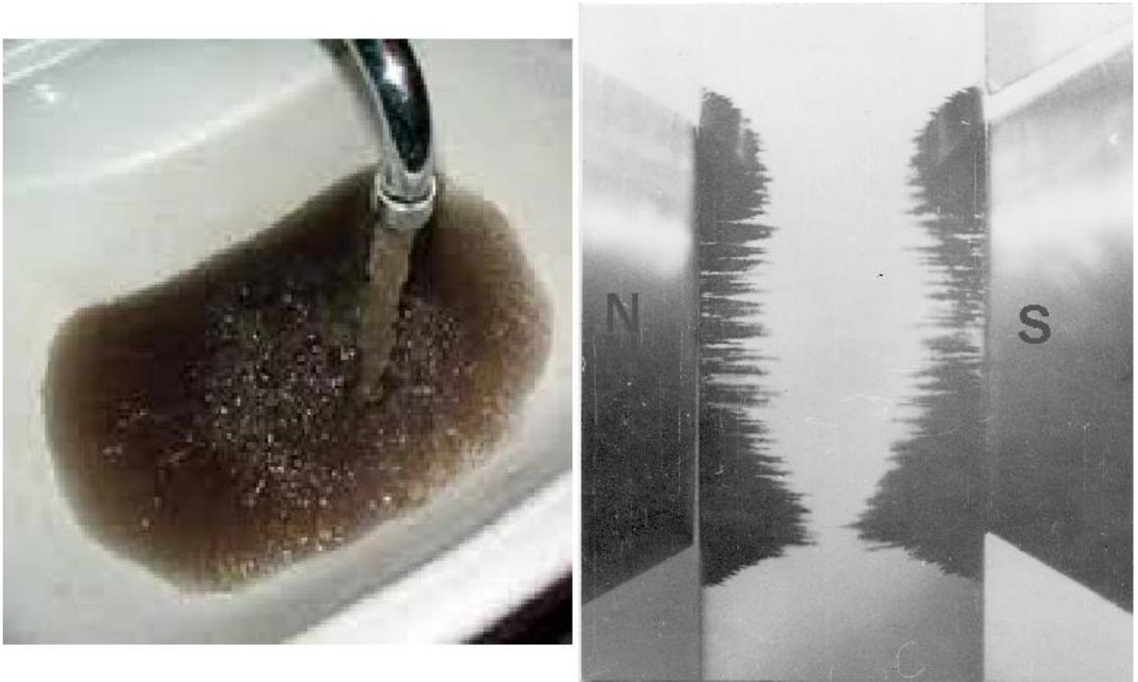
Figure 6. Photograph of the ferromagnetic admixtures filtered from passing water in the gap of electromagnetic device
